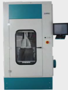
Roller Sector Compactor 30kN
